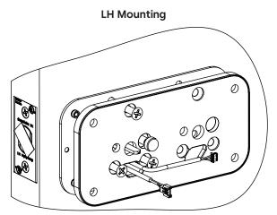
1. Harness shall be pulled gently through inside trim's backplate to accumulate all excess cables within the inside trim.
