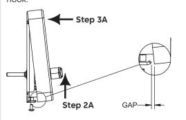
Keep clearance to min. to facilitate instal of cover
