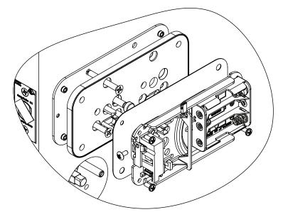
Locating post and mounting screws shall be installed as shown. Left mounting shown. Cover removed for clarity.
